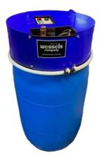
The DM-GMP unit is designed to automatically supply a pressurized solution, such as glycol and water, to a closed loop heating, chilled water, snowmelt, radiant heating, sprinkler, or process control system to ensure minimum system pressure requirements are met. These systems are equipped with HOA controls, an adjustable pressure reducing valve (PRV), pressure gauge, and a low-level alarm that cuts power to the pump and actuates an audible and visual alarm when solution levels are too low.
