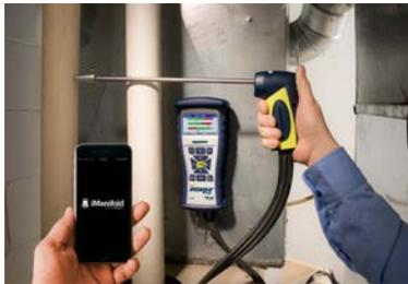
The INSIGHT Plus Combustion Analyzer collects combustion measurement data, such as oxygen and CO<sub>2</sub> concentrations, efficiency, temperature, draft and pressures, from boilers, furnaces and other heating devices. This data can now be automatically populated into the iManifold cloud reporting platform.
